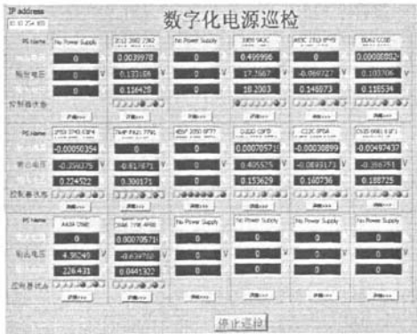
图 5 数字化电源巡检用户界面 Fig.5 Main front panel of the cyclical monitoring system of the PS.
